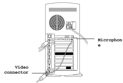
4. Plug the yellow microphone connector into the sound input port of your computer. On HP Pavilion computers, the port is marked in yellow.
